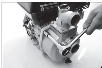
2. Remove volute and inspect for wear. Replace if eroded.
